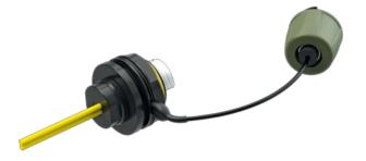
Benefiting from the expanded beam technology and the precision optical alignment the system creates high immunity against dust, mud, liquids and other contaminations. The FIBERFOX EBC25 2CH fixed patch cable connector converts a standardized LC patch cable into an expanded beam solution. It acts as a "feed-through" and has a jam-nut design
